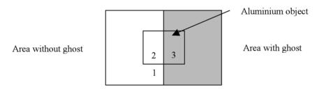
Fig. 2.2 Ghost image / erasure thoroughness measurement
