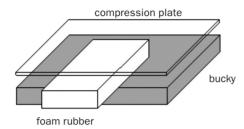
Fig. 2.5 Compression plate alignment measurement, symmetrical load
