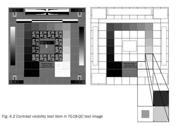
**Limiting value** All corner patches should be visible, the 5% and 95% pixel value
