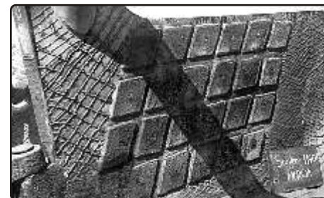
Welding Mn Steels buckets using LoTherme-457
