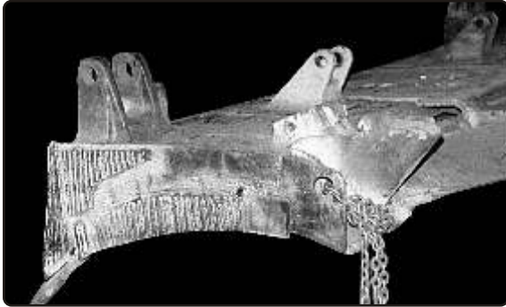
Dozer Blade hardfacing with LoTherme-604
