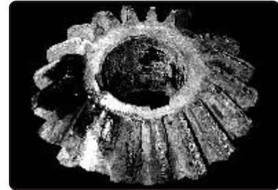
Broken gear being reclaimed with LoTherme-468
