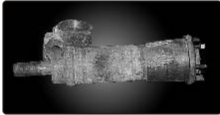
Broken Shaft Welded with LoTherme-468
