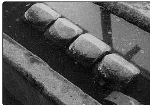
Buffer layers on work hardened Manganese steels : Recommended electrode LoTherme-610
