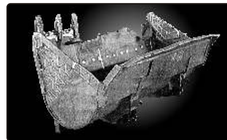
Welding heavy joints in Mn Steels : Recommended Electrode LoTherme-457
