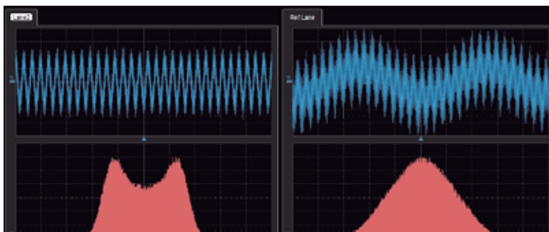
Figure 8: Examples of waveforms with periodic jitter. Left: a single periodic jitter aggressor with some random jitter mixed in. Right: both high and low frequency aggressors + random jitter.
