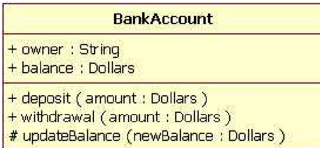
Figure 3.15: A BankAccount class that shows the visibility of its attributes and operations
