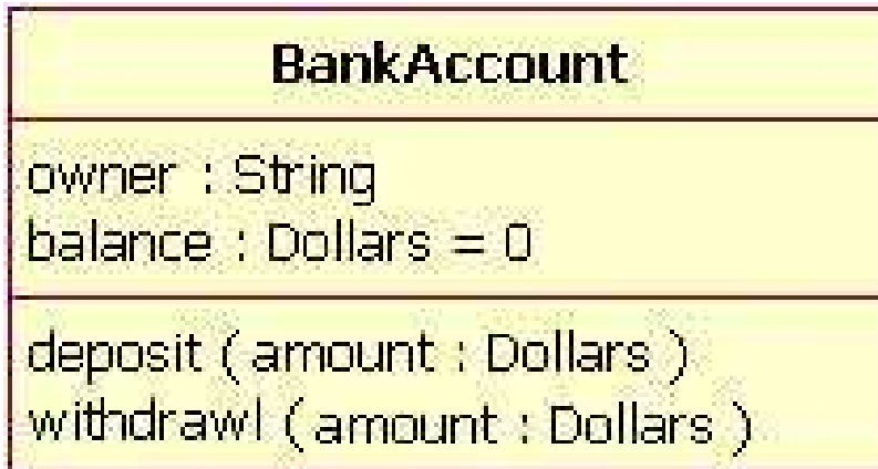
Figure 3.2: A Bank Account class diagram showing the balance attribute's value defaulted to zero dollars.
